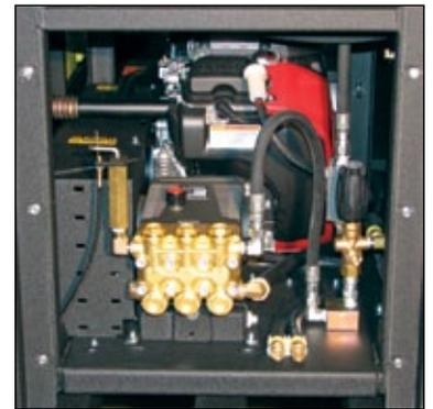
**Benefit:** The Tru-Trac Pump Rail System allows for an easy, single bolt adjustment with v-rail for alignment, and just two lockdown bolts. The Tru-Trac simplifies and assures correct pulley and belt alignment. The benefits of this feature include a decrease in belt wear and less labor cost to adjust or change belts.
