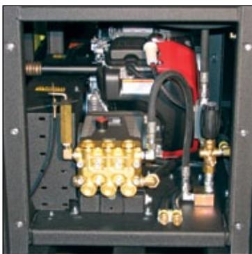
**Feature:** The unloader is an adjustable, pressure-trapping valve rated for 4,500 PSI. It's the mechanism that automatically bypasses the pump output when the operator releases the trigger on the gun and stops the flow of water. When the flow is stopped, the unloader senses the build up of
