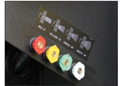
reels. Nozzles attach to the end of the wand with a quick coupler. The colors designate the spray patterns created by each nozzle: Red=0°, Yellow=15°, Green=25°, and White=40°.
