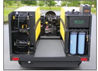
**Benefit:** The rugged frame provides protection from damage while in transit, as well as protection from being bumped while on the jobsite. The strength and durability of the frame is the result of a rectangular, rather than round, tube frame. The polyester powder coat is literally "baked" into the metal, providing all-weather protection. The frame is backed by a LANDA 7-year warranty.
