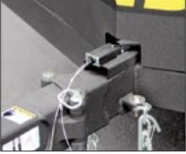
*12-V electric battery operated break-away kit not only adds additional safety but provides owners and operators peace of mind*
