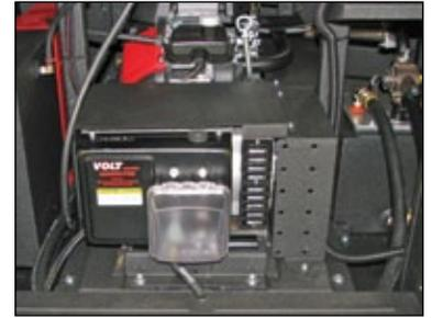
**Benefit:** The vibration isolators provide fatigue resistance by preventing the engine-pump vibration from spreading throughout the pressure washer and shaking loose nuts, bolts, electrical wiring, and burner components. This feature helps minimize maintenance, particularly on the burner assembly, and helps extend the life of the entire pressure washer.
