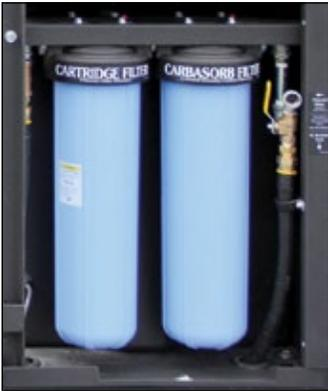
**Feature:** The integrated water reclaim and filter system recovers wash water utilizing a 120-volt vacuum turbine producing 105 CFM. A 12-volt transfer pump moves the water through a multi-stage filtration system that consists of a 50-mesh/100-micron pre-filter sock, a 20-micron pleated polyester cartridge filter, 5-micron carbon filter, and an oil absorbent media
