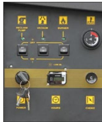
**Feature:** All system controls are conveniently placed curbside. They mounted control panel with protective and lockable cover includes a key start, choke, burner switch, adjustable thermostat, and an hour meter.
