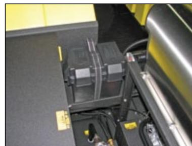
**Feature:** The 12-volt battery is located in a hardened marine-duty plastic container and placed on the ECOS platform adjacent to the heating coil (battery not included).
