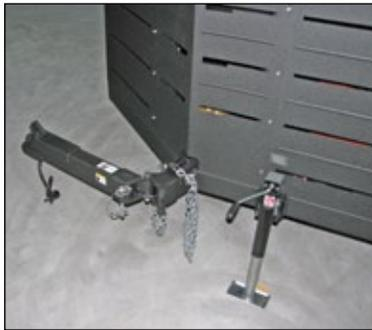
**Benefit:** The heavy-duty Swing-Away Tongue is easy to use. Simply pull the pin, swivel the tongue into position, and replace the pin. This feature allows the unit to be stowed in a small storage area. A polyester powder coating helps maximum corrosion resistance. Safety chains with lock-in, clip-on latching hooks provide additional safety as do DOT approved marker and tail lights.
