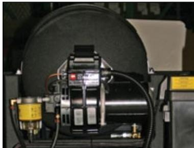
**Benefit:** Many manufacturers mount their burners under the coil and frame, making service difficult and less cost effective. However, the ECOS' horizontal coil allows the burner to be mounted at waist level with access from all sides, making burner service fast and easy. From checking the electrodes, to adjusting the air settings, the ECOS makes it simpler.
