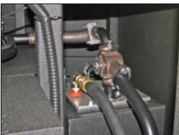
**Feature:** Patent-pending Trans-Heat Technology by LANDA. Inlet water, typically around 60°F starting in the tanks, is directed to the feed pump and received by the Trans-Heat Technology heat exchanger.
