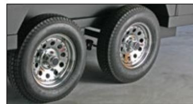
**Feature:** 205/75 tires are mounted to 15-inch chrome wheels on tandem axles with electric brakes and an industrial undercarriage leaf-spring suspension rated at 3,500 lbs. each.
