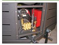
**Feature:** The open steel frame design and removable panels allow for easy access to engine and pump assembly components, including engine and pump oil drain hoses with brass plugs that lead from the engine, and pump crank cases to the edge of the platform.
