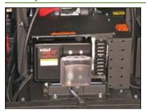
**Feature:** Heavy-duty 4,000 watt Voltmaster generator provides 120 VAC of reliable power to the burner assemblies and vacuum motor.
