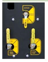
**Feature:** Tank and bypass water control valves are conveniently located in the lockable control panel cabinet on the curbside of the unit. Bypass water can be directed to either the inner or outer set of tanks. Operators can easily transport 400 gallons of water in a tandem cabinet, or they can isolate fresh water from treated water by setting the supply tank valves to separate the two 200-gallon tanks. For service
