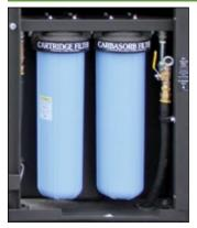
**Feature:** The integrated water reclaim and filter system recovers wash water utilizing a 120-volt vacuum turbine producing 105 CFM. A 12volt transfer pump moves the water through a multi-stage filtration system that consists of a 50-mesh/100-micron pre-filter sock, a 20-micron pleated polyester cartridge filter, 5-micron carbon filter, and an oil absorbent media
