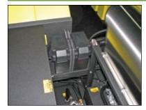
**Feature:** The 12-volt battery is located in a hardened marine-duty plastic container and placed on the ECOS platform adjacent to the heating coil (battery not included).
