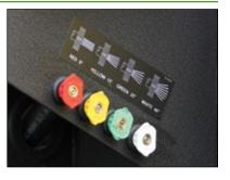
reels. Nozzles attach to the end of the wand with a quick coupler. The colors designate the spray patterns created by each nozzle: Red=0°, Yellow=15°, Green=25°, and White=40°.
